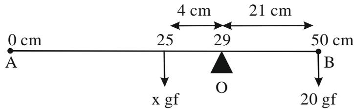
(ii) Anti-clockwise moment (ACWM) =  $x \times 4$  gf cm Clockwise moment (CWM) =  $20 \times 21$  gf cm in equilibrium, the weight of the half metre rule is 105 gf
