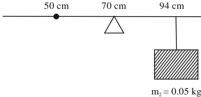
(b) As the given meter scale is a uniform scale. So, its centre of gravity lies at 50 cm. Let mass of meter scale be  $W_1$  kg.
